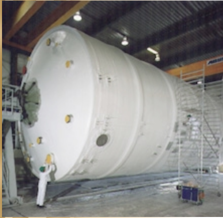
The winding machine at Plasticon Haven, one of the world's biggest in a production facility. The product being manufactured is a dual laminate polypropylene/FRP wastewater storage tank for the Sandoz chemical plant in Switzerland.
